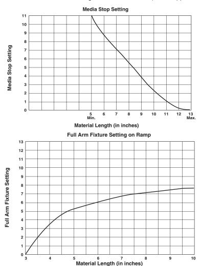
The top chart is used to determine the setting for the media stop dependent on the length of the material. The bottom chart is used to determine the setting for the full arm fixture dependent on the length of the material.
